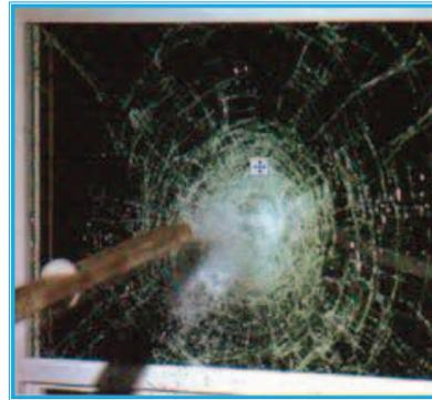
By using strategically placed reinforcement within the sash chambers along with utilizing specific hardware requirements, the Evolutions Window can now be used for impact markets
