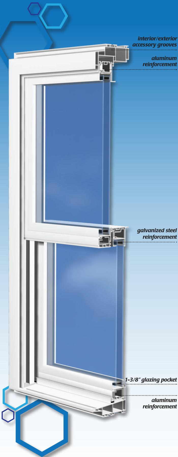
VEKA understands that field mulling, or in-house mulling of commercial windows is critical to the long term successful performance of a commercial product. We encourage the use of existing aluminum mulling profiles (thermally broken H mull or 3 piece mull) in conjunction with the Evolutions system. The evolutions frame is 3-1/4" in depth which matches most aluminum window frame configurations.
